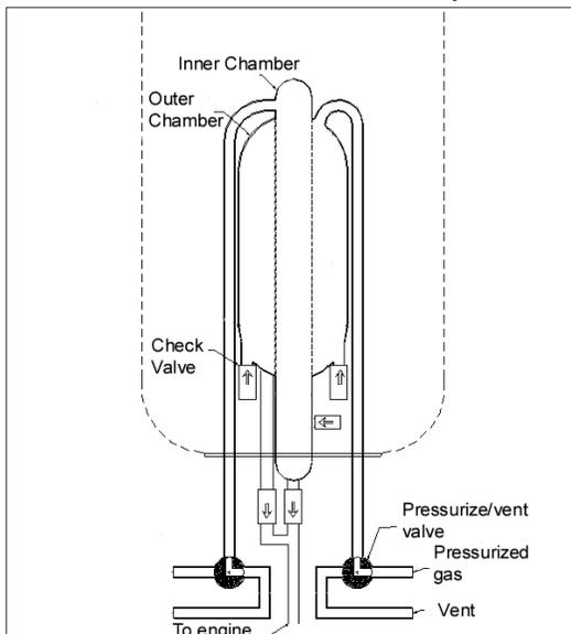
Figure 2 Prototype optimized pump design
