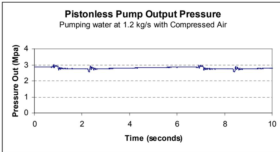
Figure 5 Prototype pump output.
