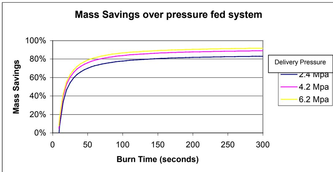
Figure 4: Mass savings as a function of burn time and delivery pressure.
