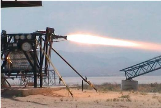
Figure 7 Atlas vernier engine running with fuel pumped and LOX pressure-fed.
